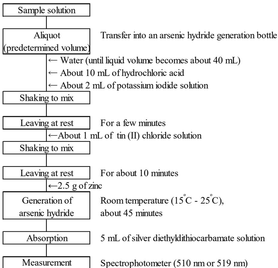
Figure 2 Flow sheet for arsenic in fertilizers
