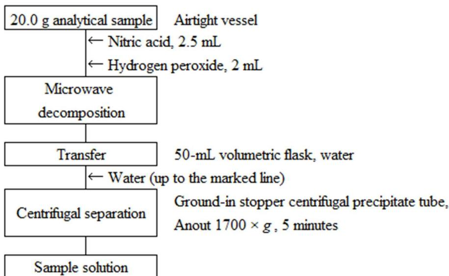
Figure 1 Flow sheet for chromium in fluid sludge fertilizers
