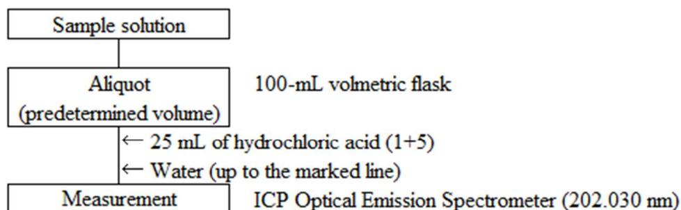
Figure 2 Flow sheet for water-soluble molybdenum in fluid fertilizers
