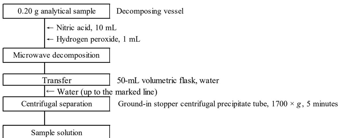
Figure 2 Flow sheet for cadmium in fertilizers except fluid sludge fertilizers (Extraction procedure)
