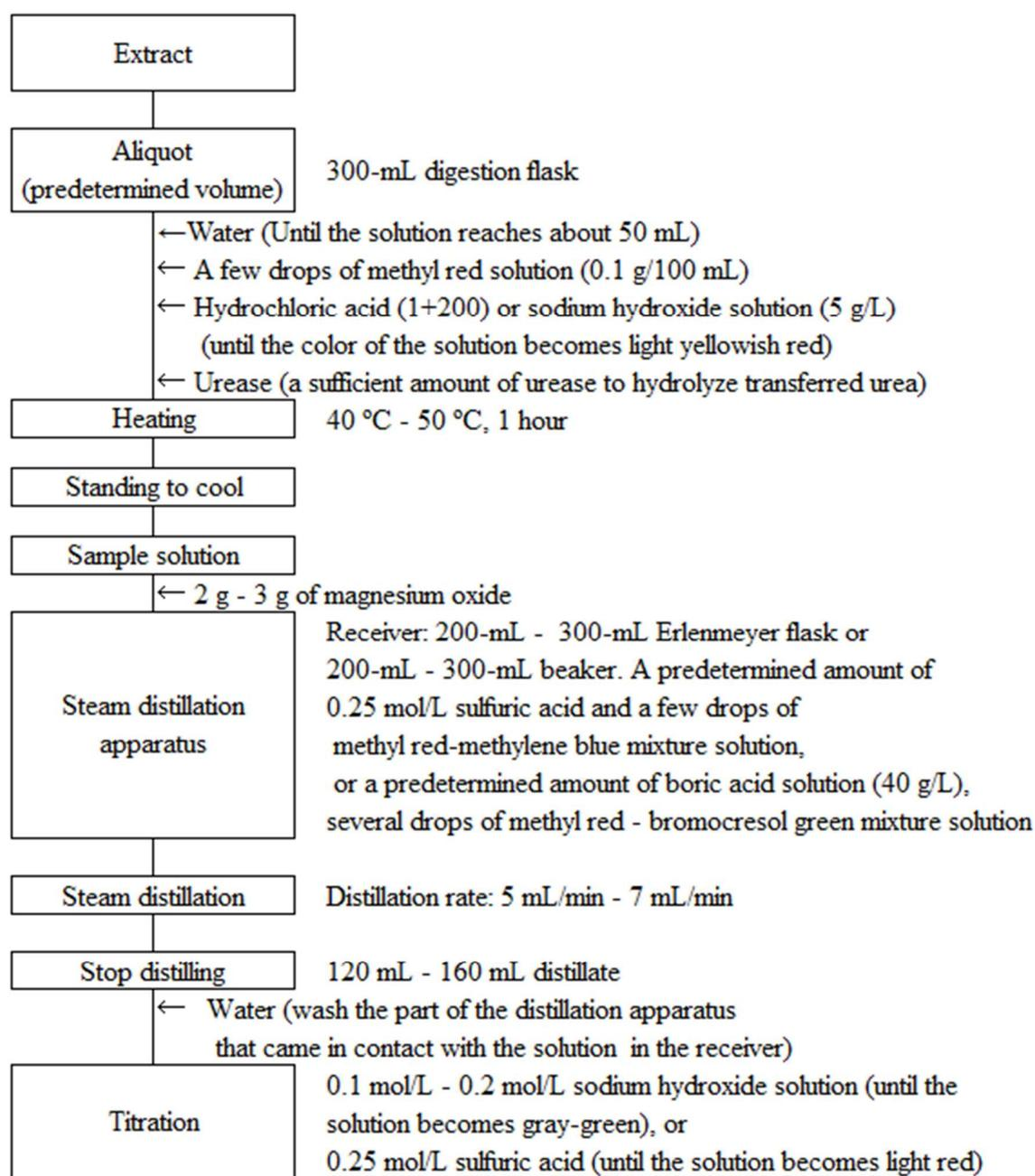
Figure 2 Flow sheet for urea nitrogen
