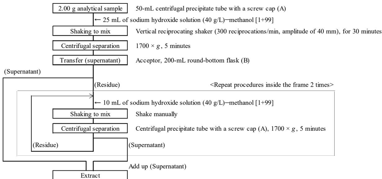
Figure 2-1 Flow sheet for clopyralid in compost and composted sludge fertilizers (Extraction procedure)
