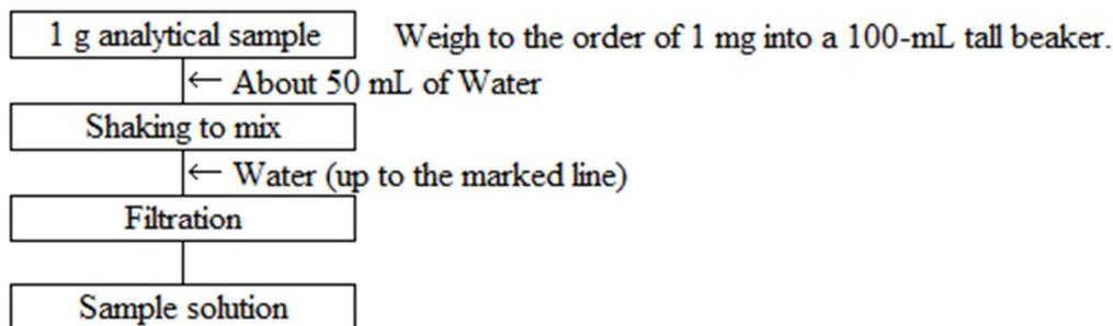
Figure 1-2 Flow sheet for water-soluble boron in fertilizers
