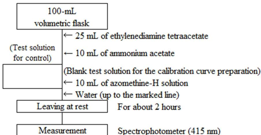
Figure 2-3 Flow sheet for water-soluble boron in fertilizers
