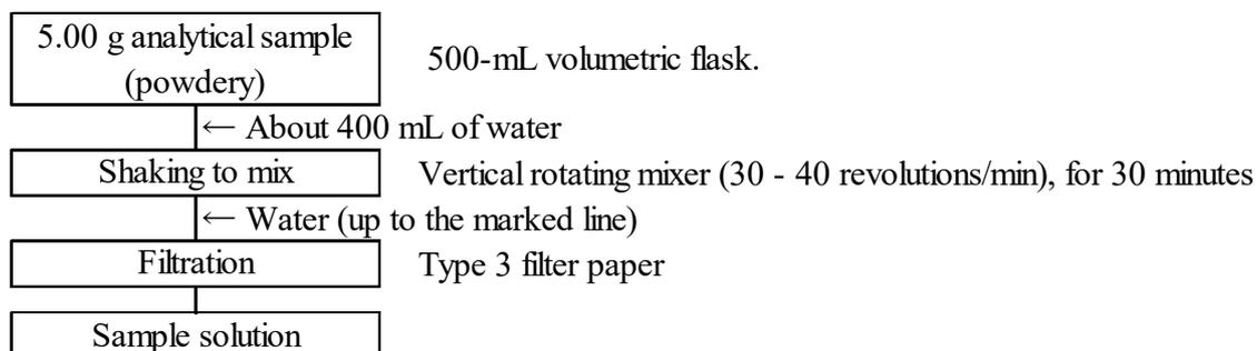
Figure 1-1 Flow sheet for water-soluble molybdenum in fertilizers (Extraction procedure (4.1.1))
