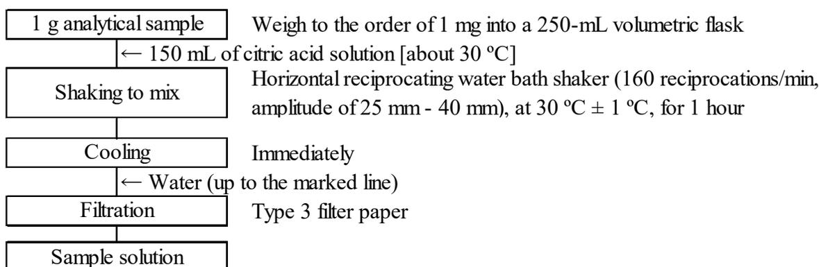
Figure 1-2 Flow sheet for citric acid-soluble boron in fertilizers (Extraction procedure (4.1.2))
