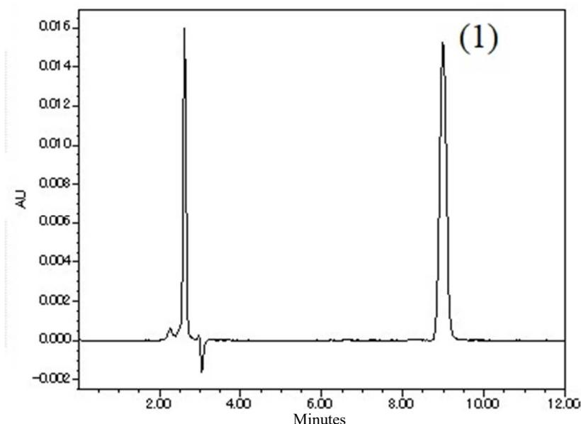
Reference diagram: HPLC chromatogram of the standard solutions for calibration curb preparation (10 mg/L)
