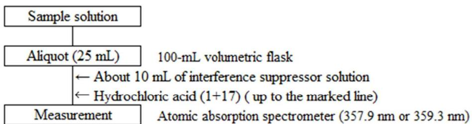
Figure 2 Flow sheet for chromium in calcined sludge fertilizer and fertilizers not containing organic matters (Measurement procedure)
