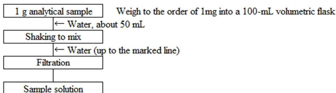
Figure 1 Flow sheet for water-soluble molybdenum in fluid fertilizers
