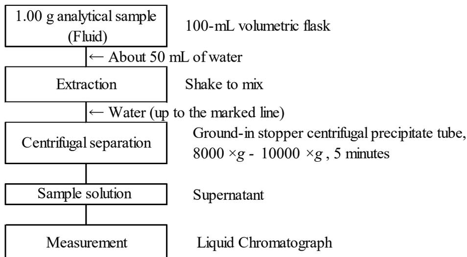
Figure 2 Flow sheet for guanylurea nitrogen in fertilizers (Extraction procedure (4.1.2) and measurement)
