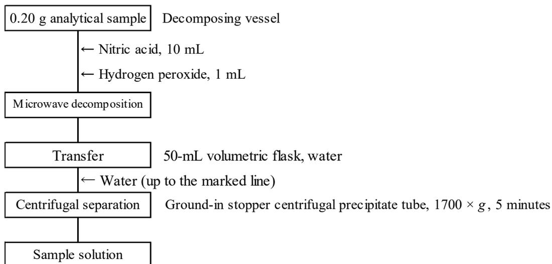
Figure 2 Flow sheet for lead in fertilizers except fluid sludge fertilizers (Extraction procedure)
