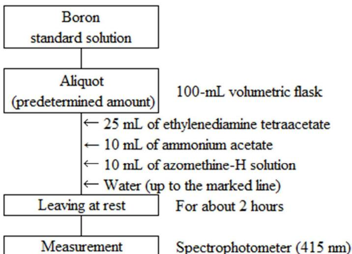
Figure 2-2 Flow sheet for water-soluble boron in fertilizers (Preparation and measurement procedures of boron standard solution for the calibration curve preparation)
