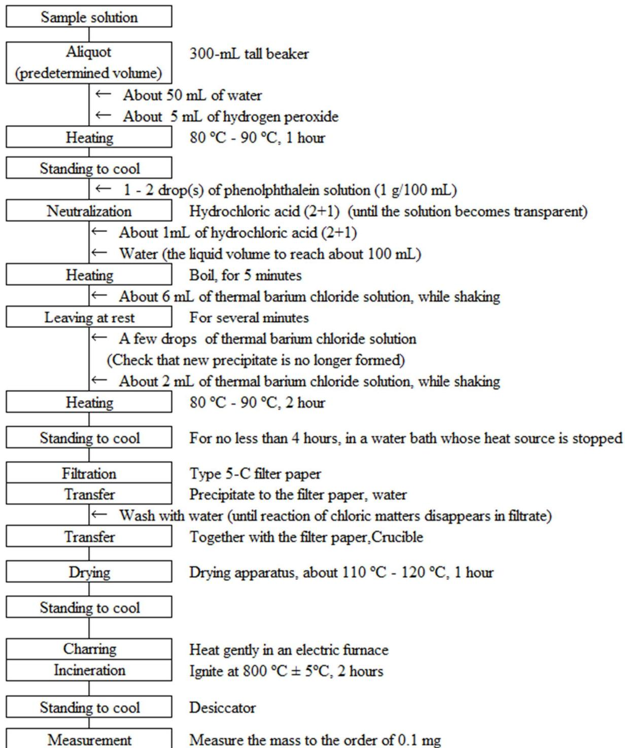
Figure 2 Flow sheet for total sulfur content in fertilizers
