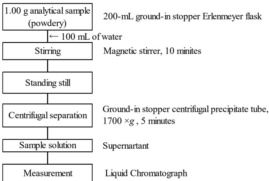
Figure 1 Flow sheet for biuret nitrogen in fertilizers
