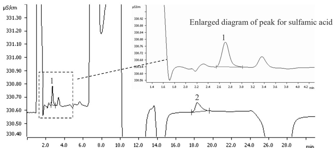
(B) Sample solution (the equivalents of 0.25 % (mass fraction) (2500  $\mu$ g/g) as sulfamic acid and ammonium thiocyanate added in ammonium sulfate, respectively)
