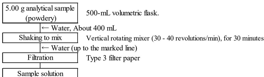
Figure 1-1 Flow sheet for water-soluble copper in fertilizers (Extraction procedure (4.1.1))
