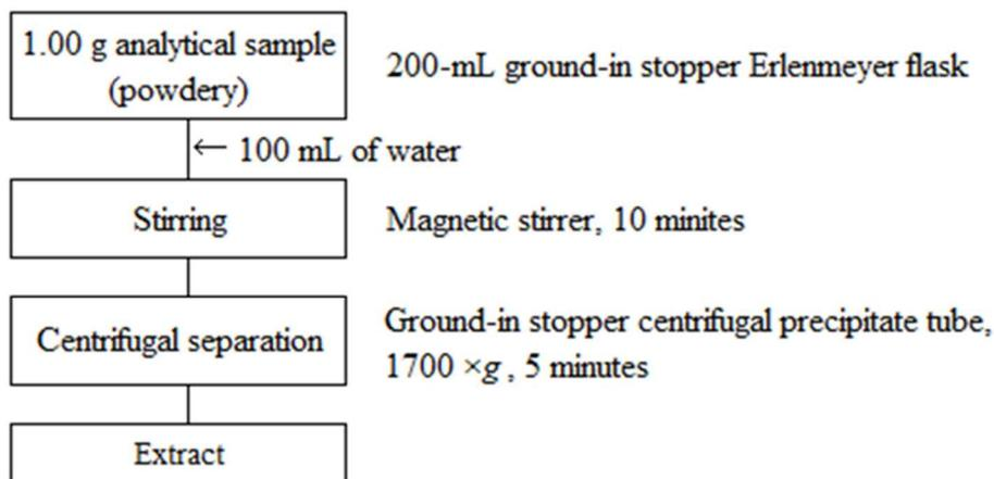
Figure 1-1 Flow sheet for sulfamic acid in fertilizers
