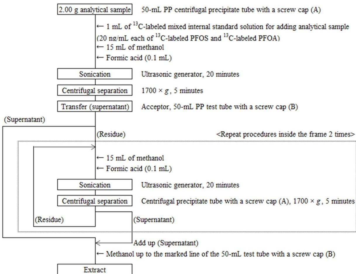
Figure 2-1 Flow sheet for organofluorine compounds in sludge fertilizers (Extraction procedure)
