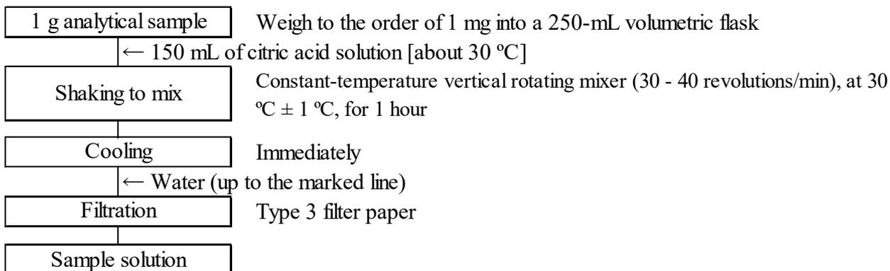
Figure 1-1 Flow sheet for citric acid-soluble boron in fertilizers (Extraction procedure (4.1.1))
