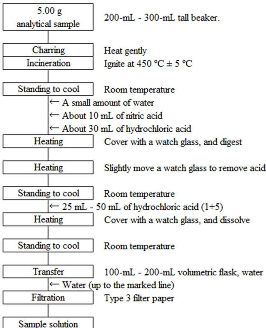
Figure 1 Flow sheet for cadmium in sludge fertilizers
