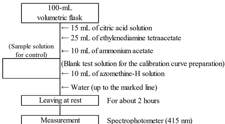
Figure 2-3 Flow sheet for citric acid-soluble boron in fertilizers
