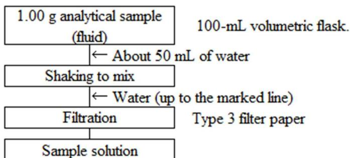
Figure 1-2 Flow sheet for water-soluble molybdenum in fertilizers (Extraction procedure (4.1.2))
