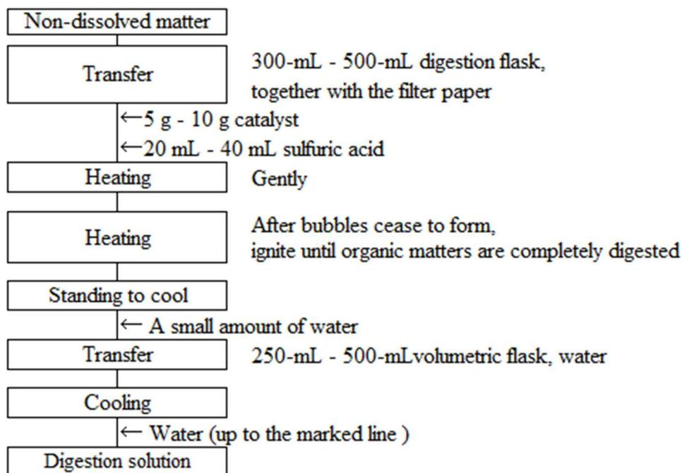
Figure 2 Flow sheet of the testing method for heat buffer solution soluble nitrogen in methyolurea polymerization fertilizers ( Kjeldahl digestion procedure)
