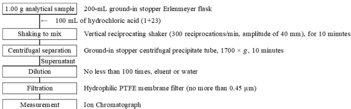
Figure Flow sheet for acid-soluble sulfur in fertilizers
