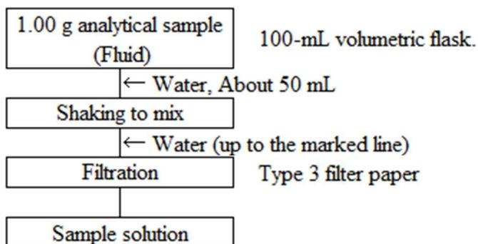
Figure 1-2 Flow sheet for water-soluble iron in fertilizers
