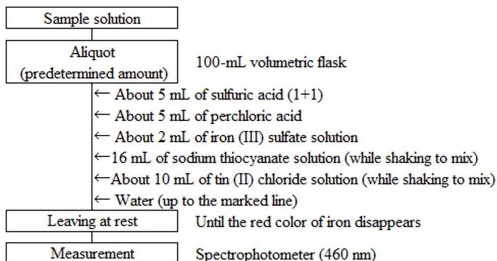
Figure 2 Flow sheet for water-soluble molybdenum in fertilizers (Measurement procedure)
