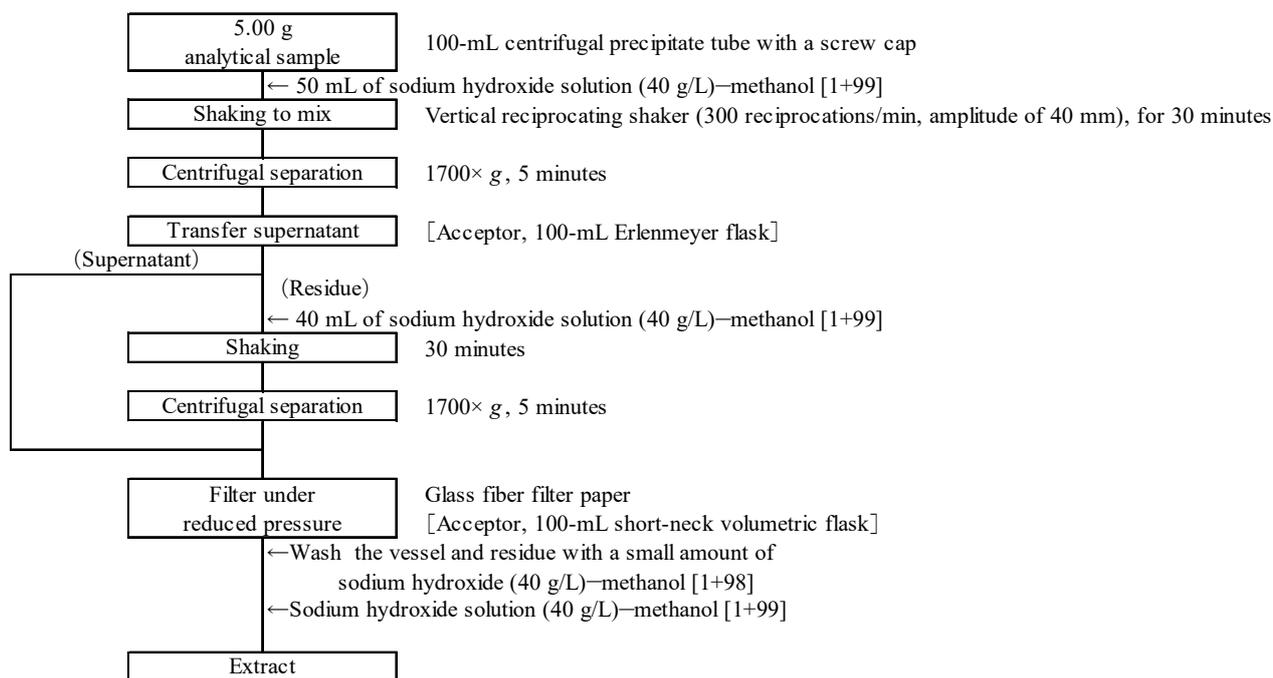
Figure 1 Flow sheet for clopyralid in compost and composted sludge fertilizers (Extraction procedure)
