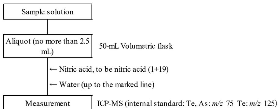
Figure 3 Flow sheet for arsenic in fertilizers (Measurement procedure)
