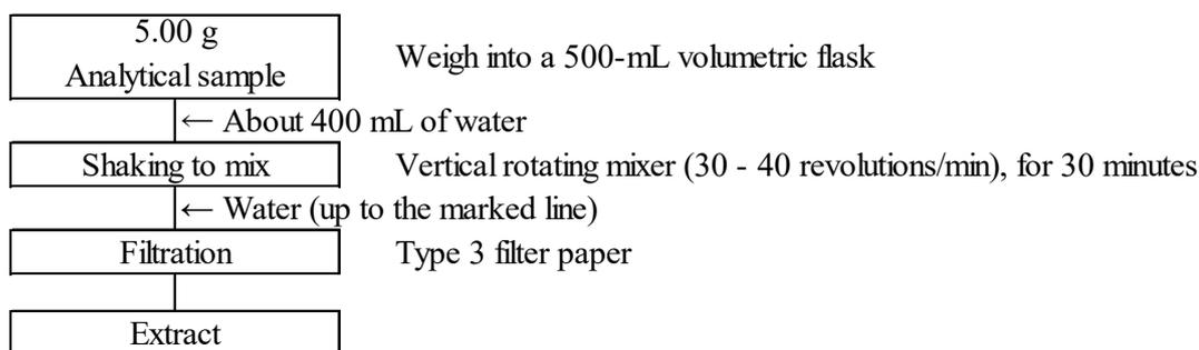
Figure 1-1 Flow sheet for urea nitrogen
