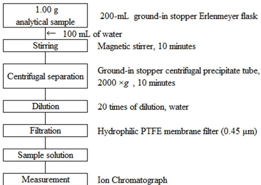
Figure Flow sheet for chlorine in fertilizers
