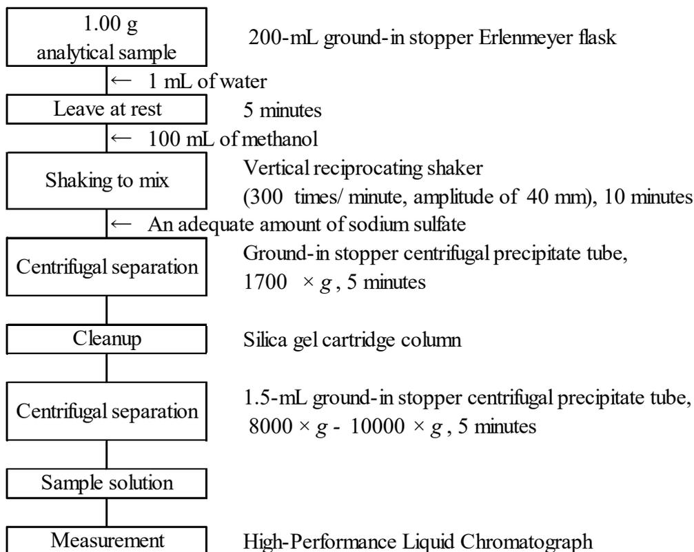
Figure Flow sheet for dicyandiamide (Dd) in fertilizers
