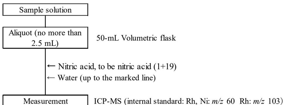
Figure 3 Flow sheet for nickel in fertilizers (Measurement procedure)
