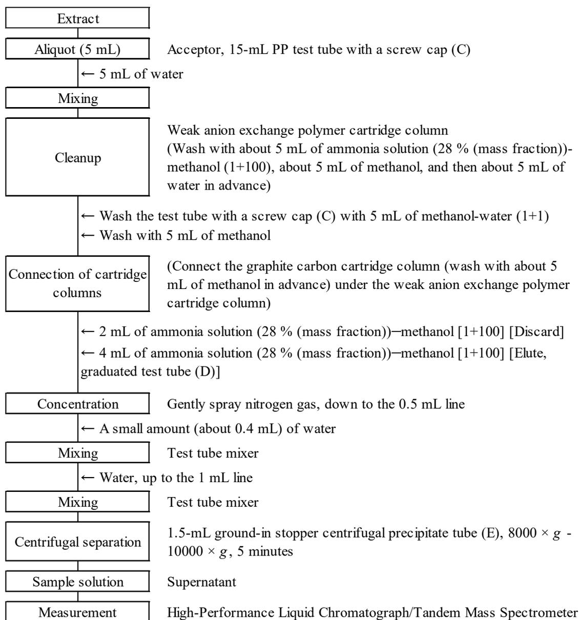
Figure 2-2 Flow sheet for organofluorine compounds in sludge fertilizers (Cleanup and measurement procedures)
