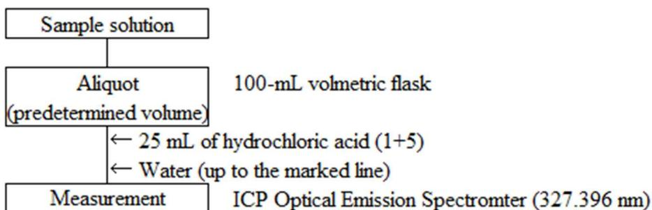
Figure 2 Flow sheet for water-soluble copper in fluid fertilizers (Measurement procedure)
