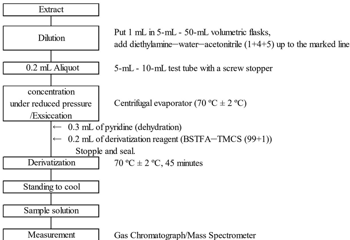
Figure 2 Flow sheet for melamine derivations in fertilizers (Derivatization and measurement procedure)
