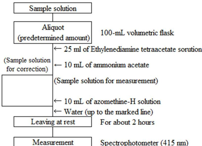
Figure 2-1 Flow sheet for water-soluble boron in fertilizers (Preparation and measurement procedures of sample solution for measurement and sample solution for correction)
