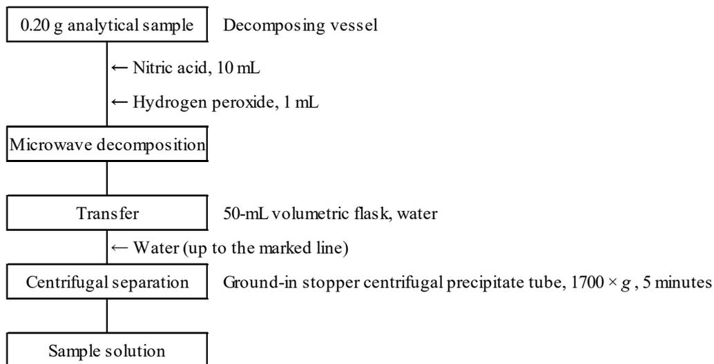
Figure 2 Flow sheet for arsenic in fertilizers except fluid sludge fertilizers (Extraction procedure)
