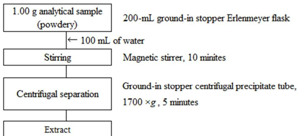
Figure 1-1 Flow sheet for nitrous acid in fertilizers (Extraction procedure (4.1.1))
