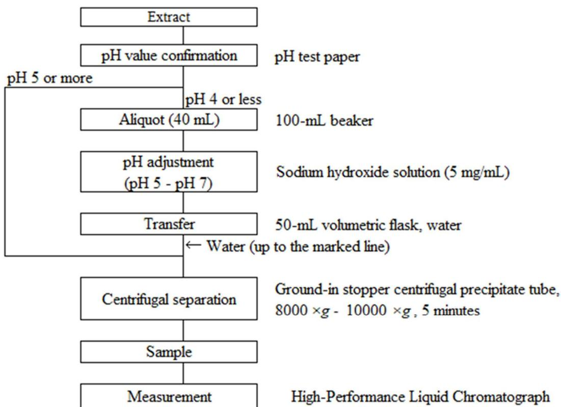
Figure 2 Flow sheet for nitrous acid in fertilizers
