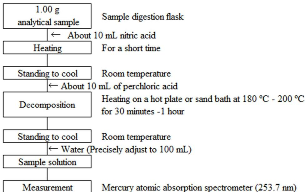
Figure Flow sheet for mercury in fertilizers
