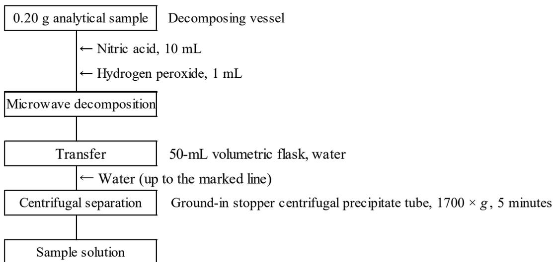
Figure 2 Flow sheet for chromium in fertilizers containing organic matters except fluid sludge fertilizers (Extraction procedure)
