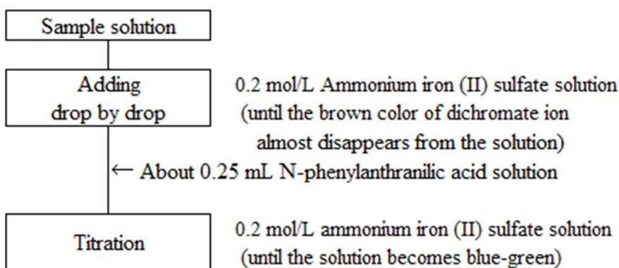
Figure 2 Flow sheet for organic carbon in sludge fertilizers and compost, etc.
