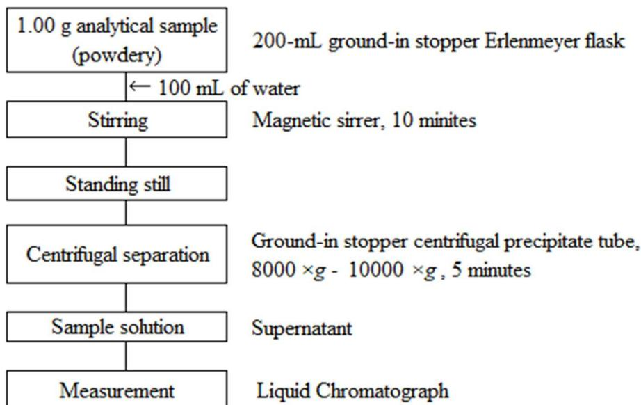
Figure 1 Flow sheet for urea nitrogen in fertilizers
