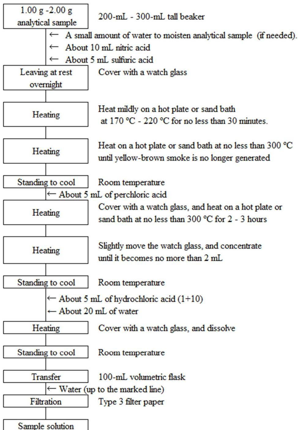
Figure 1 Flow sheet for arsenic in fertilizers (Extraction procedure)
