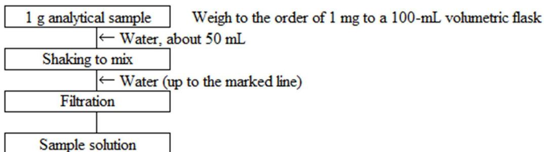
Figure 1 Flow sheet for water-soluble zinc in fluid fertilizers (Extraction procedure)
