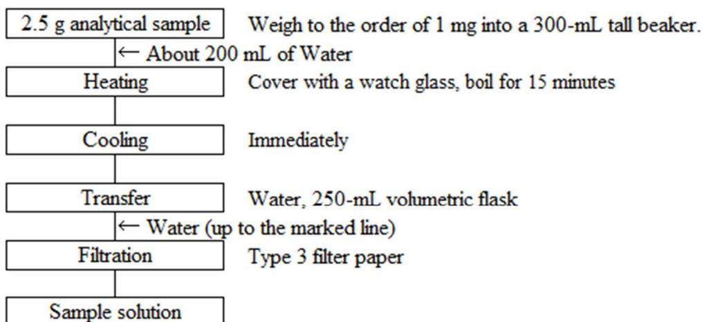
Figure 1-1 Flow sheet for water-soluble boron in fertilizers
