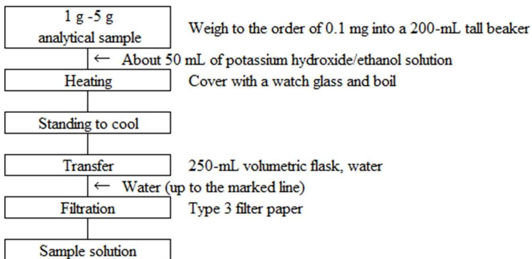
Figure 1 Flow sheet for total sulfur content in fertilizers
