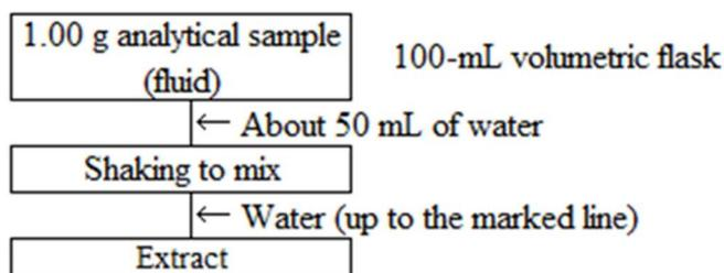
Figure 1-2 Flow sheet for sulfamic acid in fertilizers
