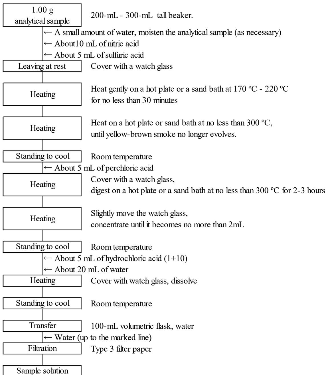
Figure 1 Flow sheet for chromium in calcined sludge fertilizer and fertilizers not containing organic matters (Extraction procedure)
