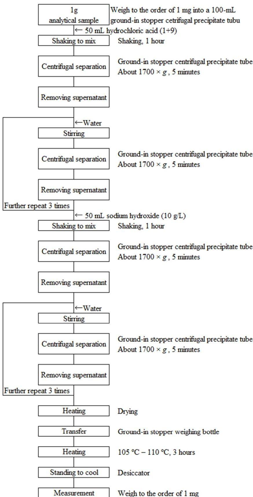
Figure 2 Flow sheet of the testing method for humic acid in humic acid salt fertilizers (Testing procedure of acid insoluble - alkali non-dissolved matter (4.2))
