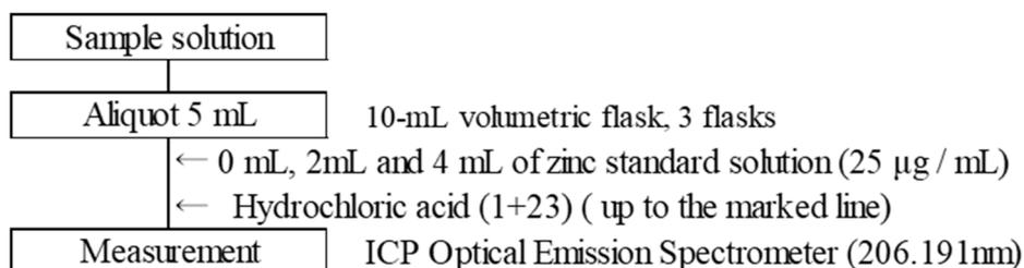
Figure 2 Flow sheet for total zinc in fertilizers (Measurement procedure)
