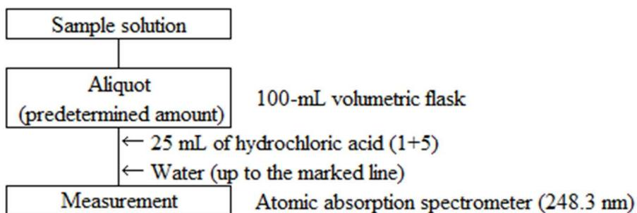
Figure 2 Flow sheet for water-soluble iron in fertilizers
