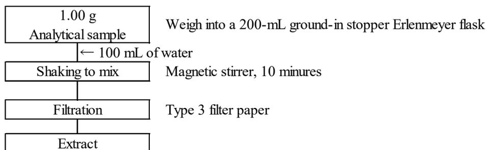
Figure 1-2 Flow sheet for urea nitrogen
