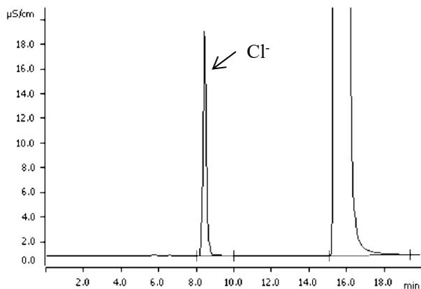
(A) Chromatogram of magnesia potassium sulfate (Suppressor method)
