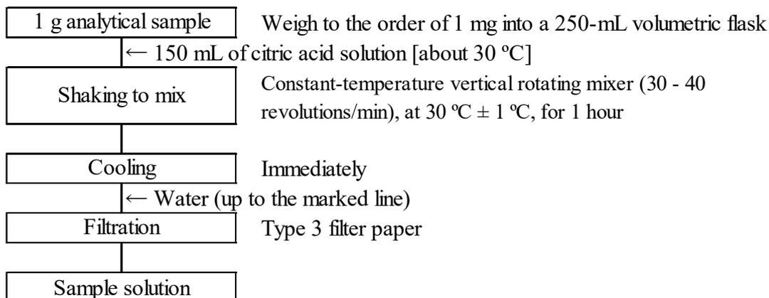
Figure 1-1 Flow sheet for citric acid-soluble boron in fertilizers
