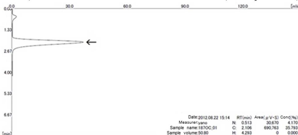
2) Total carbon in an analytical sample (sludge fertilizer)
