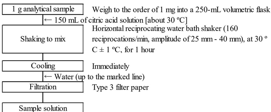
Figure 1-2 Flow sheet for citric acid-soluble boron in fertilizers
