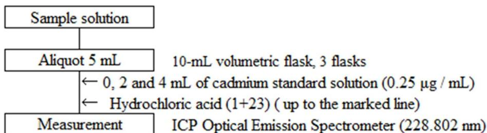
Figure 2 Flow sheet for cadmium in sludge fertilizers
