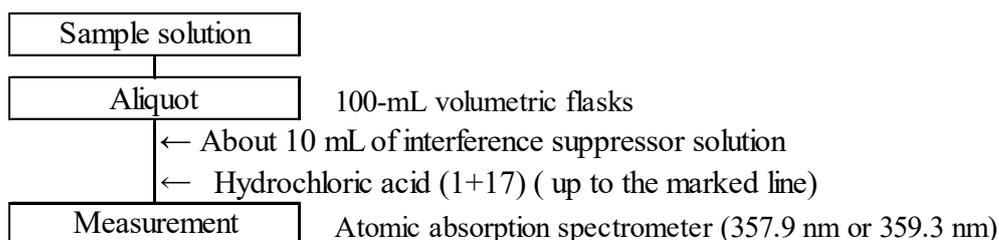
Figure 2 Flow sheet for chromium in fertilizers mainly containing fused matters and slag, etc. (Measurement procedure)
