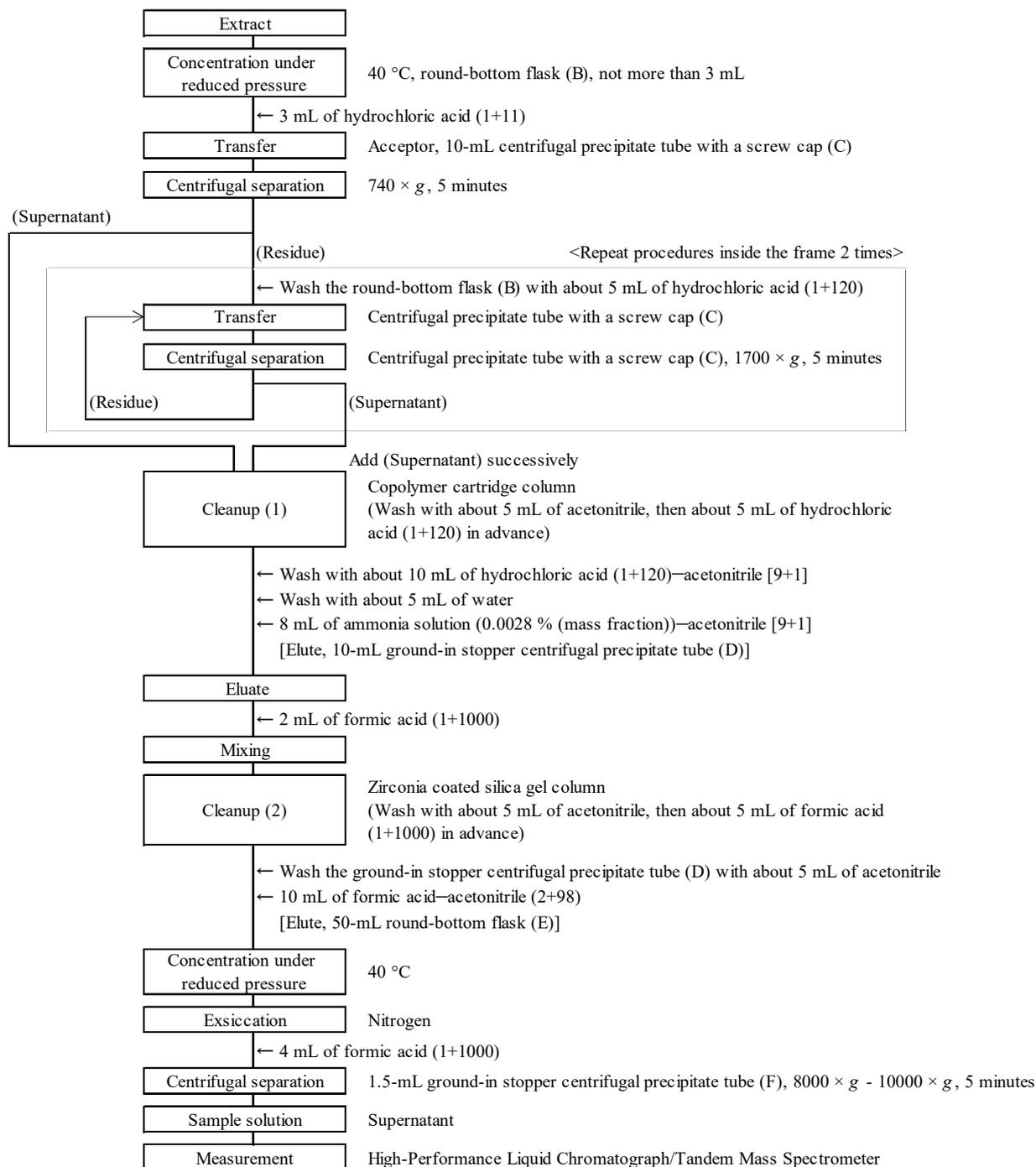
Figure 2-2 Flow sheet for clopyralid in compost and composted sludge fertilizers (Cleanup (1), cleanup (2) and measurement procedures)
