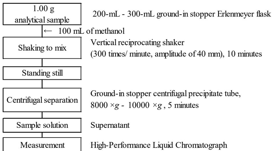
Figure Flow sheet for dicyandiamide nitrogen in nitrolime and fertilizers containing nitrolime
