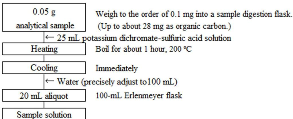
Figure 1 Flow sheet for organic carbon in sludge fertilizers and compost, etc.
