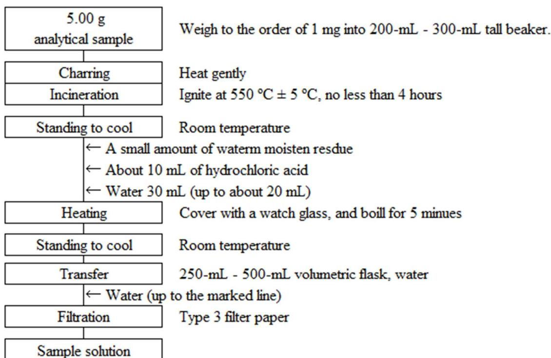
Figure 1-1 Flow sheet for total copper in fertilizers
