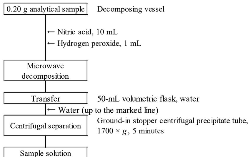
Figure 2 Flow sheet for nickel in fertilizers except fluid sludge fertilizers (Extraction procedure)
